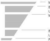
Multiple pigment coating Bleached chemical pulp + Unprinted PIW Mechanical pulp
